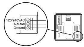
Figure 3.13 90-260 VAC Instrument Power Connections
